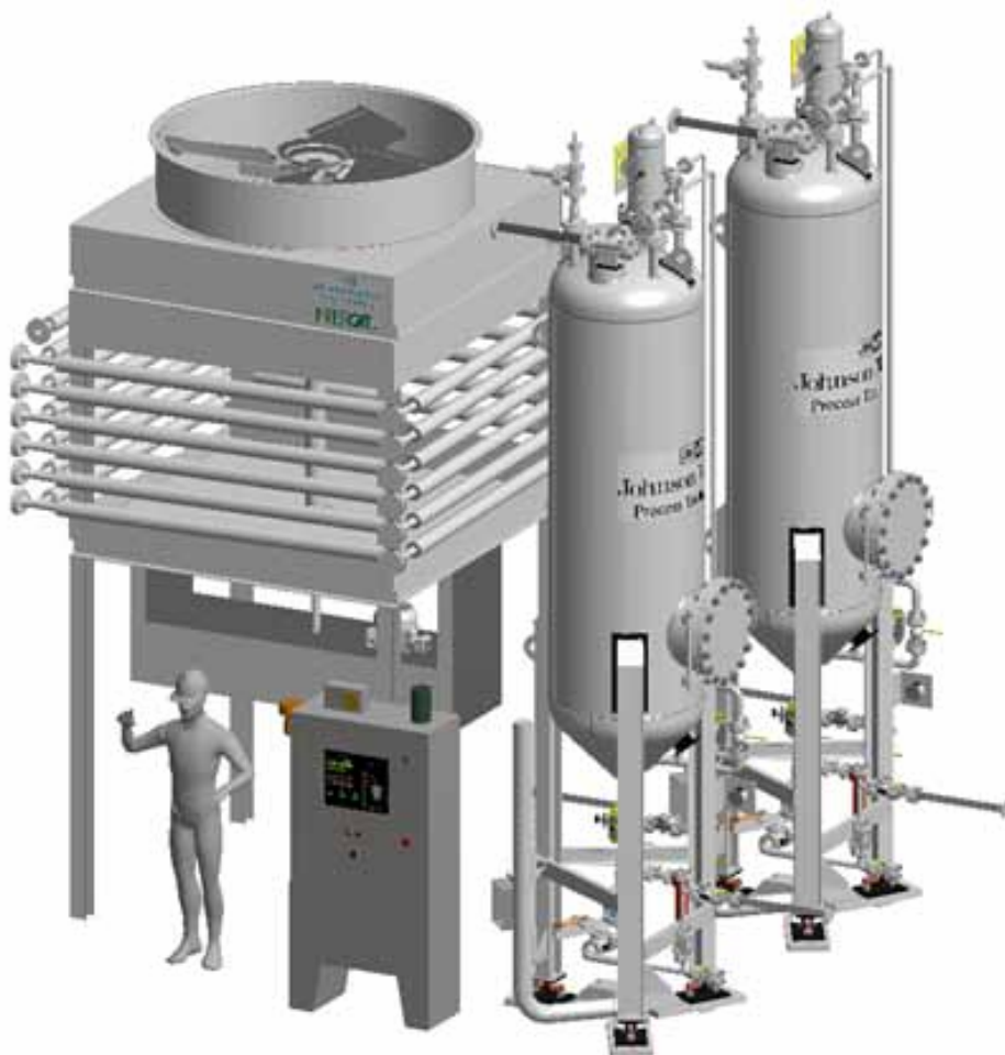
Image 3 – Mark-II Design Continuous Catalyst Withdrawal System
