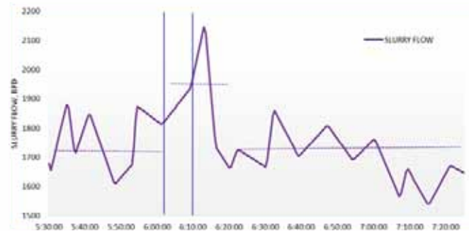
Chart 5 – US Refiner 1: Batch Catalyst Withdrawal (Impact on Slurry Yield) 2
