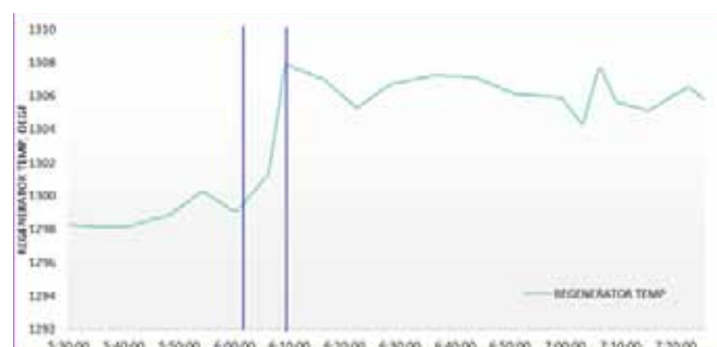
Chart 2 - US Refiner 1: Batch Catalyst Withdrawal (Regenerator Temperature) 2
